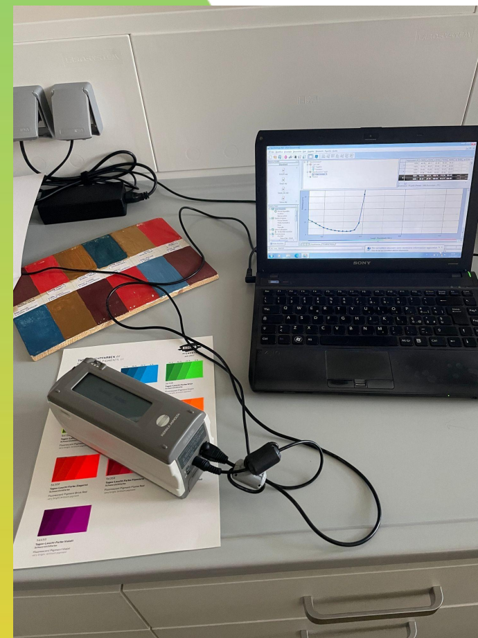
Colorimetro collegato al computer
